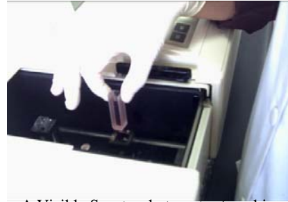
A Visible Spectrophotometer (machine pictured) is used to read Vitamin C concentration from liquefied potato
